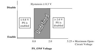
Figure 8. PS\_ON# Signal Characteristics
